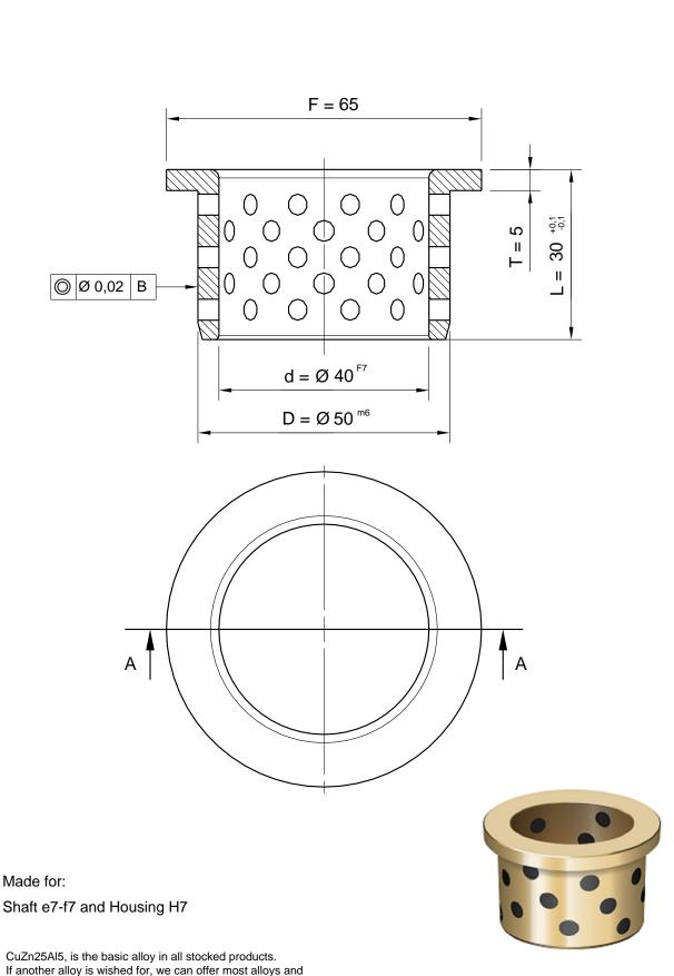
CuZn25Al5, is the basic alloy in all stocked products. If another alloy is wished for, we can offer most alloys and special sizes acc. to your requirements.
